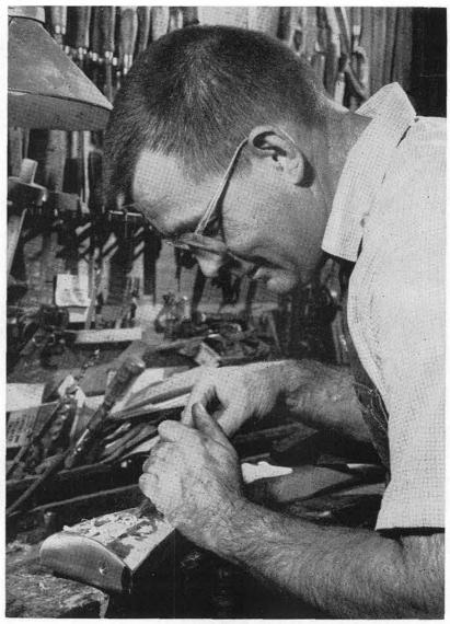
CAREFUL inletting and detail work is characteristic of Hicks muzzle-loading rifles. Here, Dick routs out patch-box cavity in a partially-finished stock. Some models require over 400 hours work.
